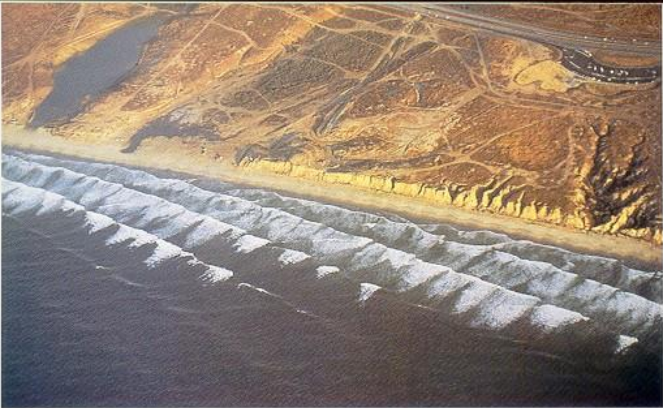
FIGURE 13.12 Waves arriving obliquely onshore along a coast near Oceanside, California, change orientation as they encounter the bottom and begin to slow down. As a result, each wave front is refracted so that it more closely parallels the bottom contours. The arriving waves develop a longshore current that moves from left to right in this view.
