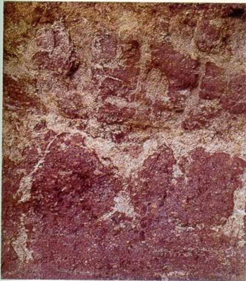
FIGURE B7.1 Red, iron-rich laterite near Khao Yai, Thailand. Originally a conglomerate, the rock is now a mixture of limonite and clay as a result of extreme tropical leaching.
