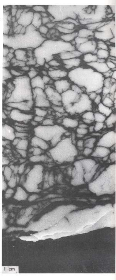
FIGURE 8.2 Chickenwire structure in anhydrite. Evaporite series of the Lower Lias (Jurassic), Aquitaine Basin, southwest France. (From Bouroullec, J., 1981, Sequential study of the top of the evaporitic series of the Lower Lias in a well in the Aquitaine Basin (Auch 1), southwestern France, in Chambre Syndical de la Recherche et de la Production due Pétrole et du Gaz Naturel (eds.), Evaporite deposits: Illustration and interpretation of some environmental sequences , Pl. 36, p. 157, reprinted by permission of Editions Technip, Paris, and Gulf Publishing Co., Houston, Tx. Photograph courtesy of J. Bouroullec.)
