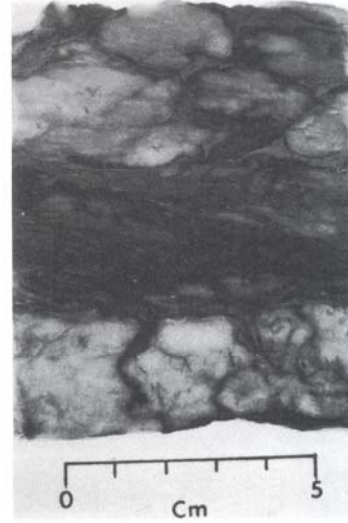
FIGURE 8.1 Nodular anhydrite in a core sample of the Buckner Anhydrite (Jurassic), Texas. Dark-colored carbonate separates and surrounds the lighter-colored anhydrite nodules.
