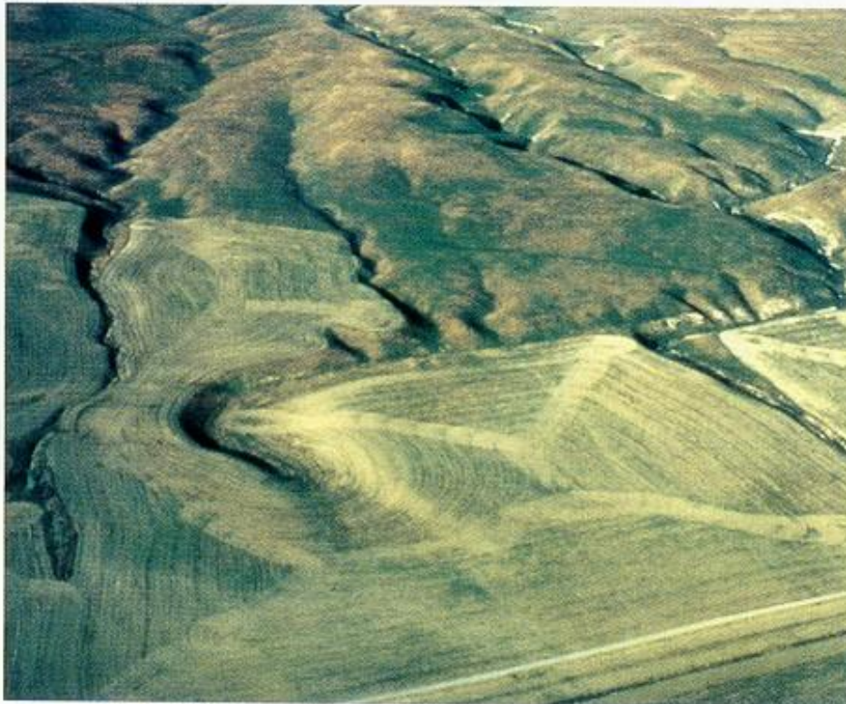
Figure 20.20 The San Andreas Fault , in California, is a major strike-slip fault. It is delineated by prominent, straight ridges and valleys. Recent movement along the fault has offset the drainage patterns on either side of the fault. Relative movement between the fault blocks is evident from the direction in which the drainage is offset.
