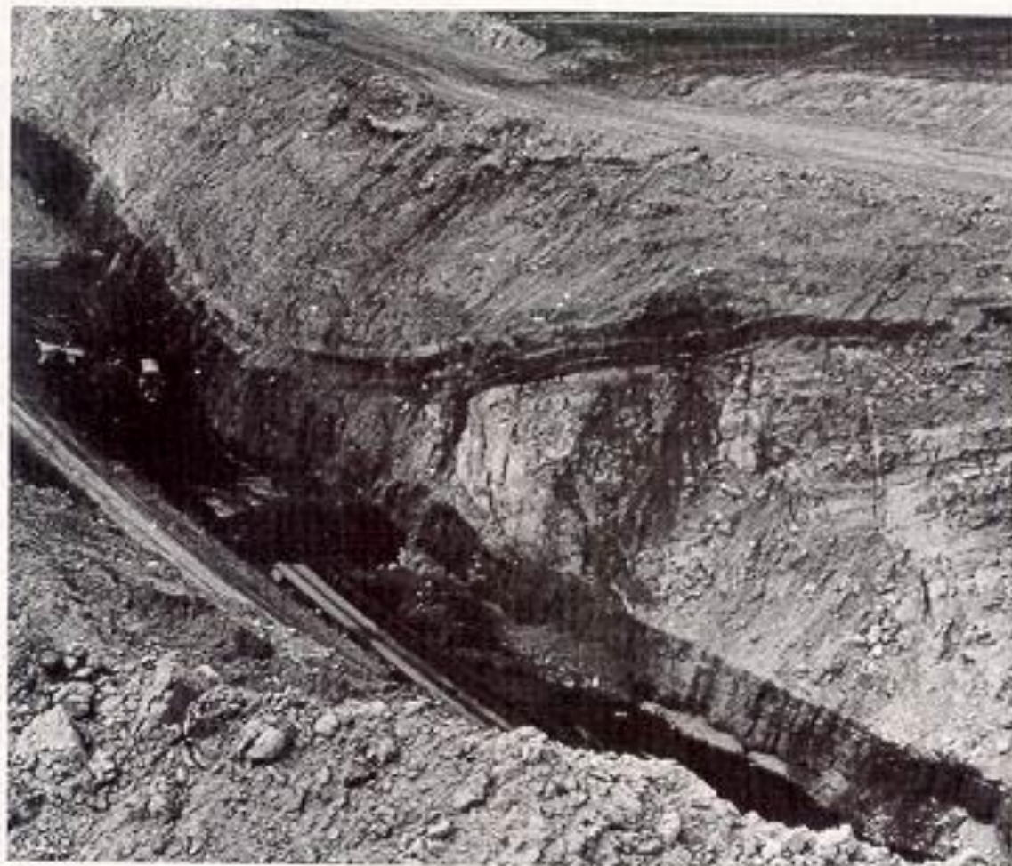
Fig. 5.4 Zig-zag split in coal seam, New South Wales, Australia. The uppermost seam is visible near the top of the highwall, and joins the split to the right of the photograph.
