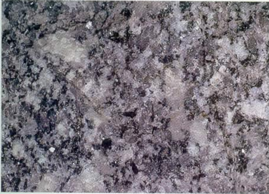
Figure 3.2 A. Close-up of interlocking crystals in a coarse-grained igneous rock. The largest crystals are about 1 centimeter in length. B. Photomicrograph of interlocking crystals in a coarse-grained igneous rock. (Photos by E.J. Tarbuck)
