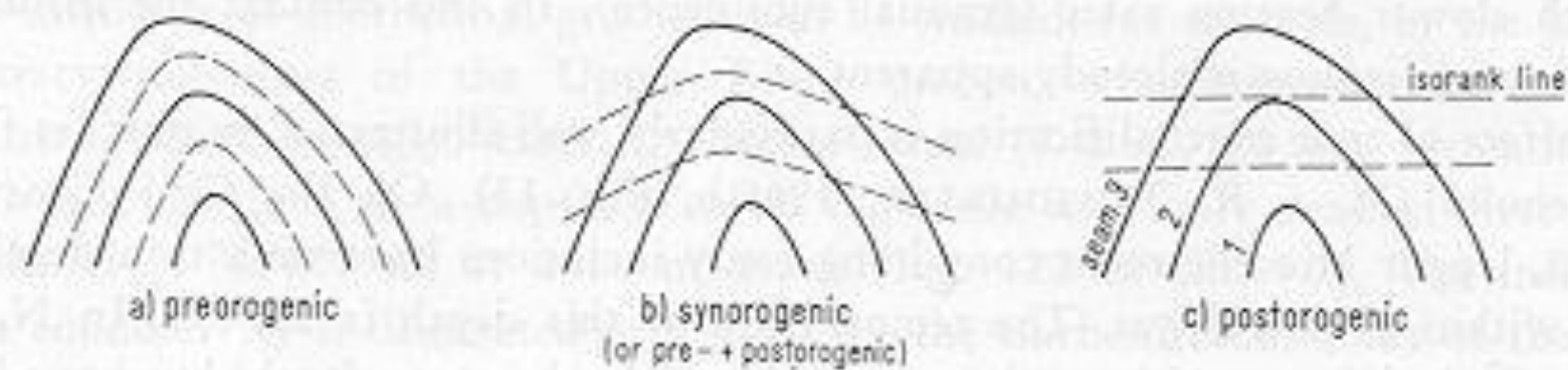
Fig. 21. Course of isorank lines (e. g. isovols, isorefectances) in cross-sections of a folded area after a) preorogenic; b) synorogenic and c) postorogenic coalification (after M. & R. TEICHMÜLLER, 1966 a).
